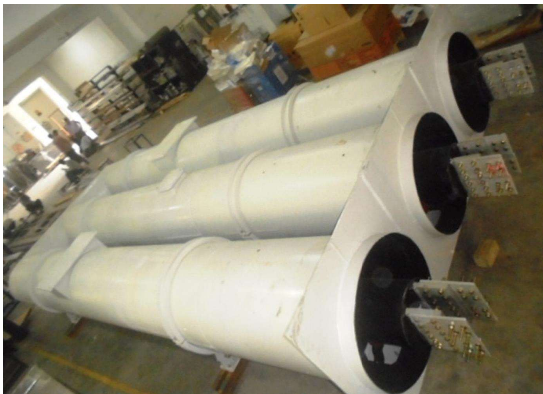
Isolated Phase Bus duct
